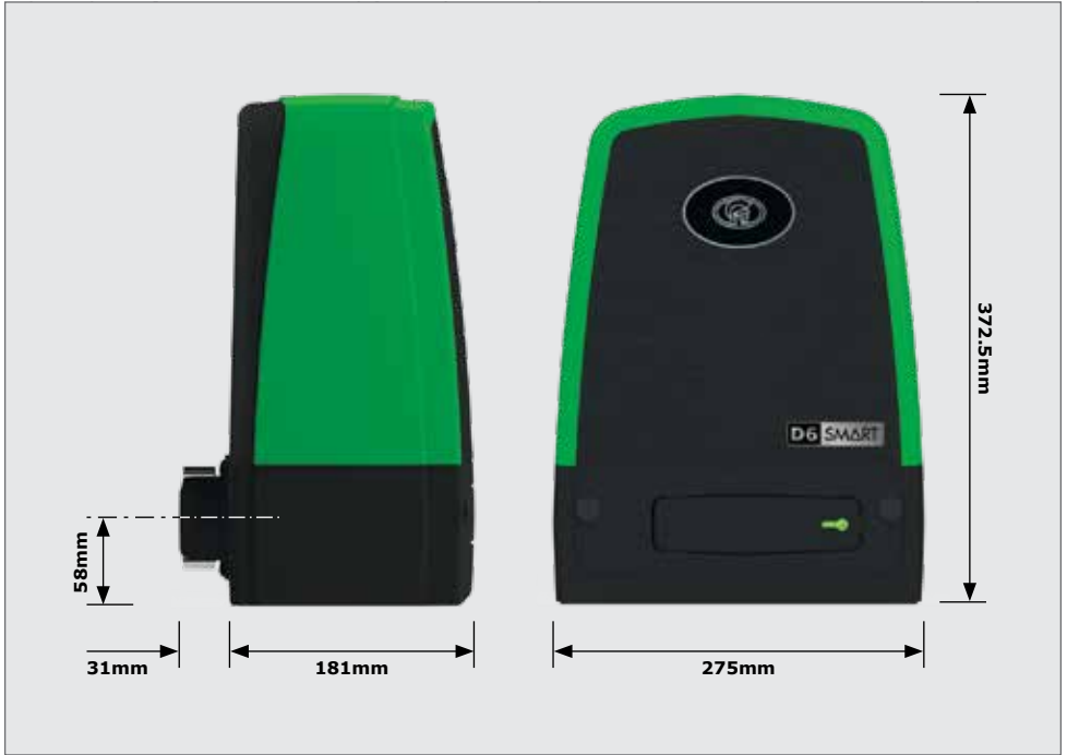
FIGURE 1. D6 SMART PHYSICAL DIMENSIONS
